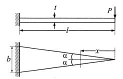
Q.52 The area moment of inertia about the neutral axis of a cross-section at a distance x measured from the free end is
