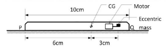
Given in addition that the eccentric mass = 2 grams, eccentricity = 2.19 mm, mass of the mobile = 90 grams,  $g = 9.81 \text{ m/s}^2$ . Uniform speed of the motor in RPM for which the mobile will get just lifted off the ground at the end Q is approximately
