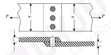
width of the plate w = 200 mm, thickness of the plate t = 5 mm, number of rivets n = 3, diameter of the rivet  $d_r = 10 \text{ mm}$ , diameter of the rivet hole  $d_h = 11 \text{ mm}$ , allowable tensile stress of the plate  $\sigma_p = 200 \text{ MPa}$ , allowable shear stress of the rivet  $\sigma_s = 100 \text{ MPa}$  and allowable bearing stress of the rivet  $\sigma_c = 150 \text{ MPa}$ .
