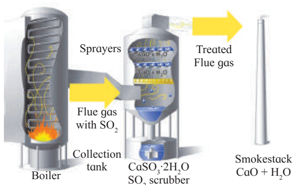
Fig. 15.5 : Exhaust gas Scrubber
