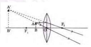
The above lens has a focal length of 10 cm. The object of height 2 mm is placed at a distance of 5 cm from the pole. Find the height of the image.
