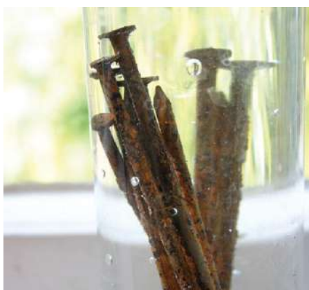
Fig. 6.5 Rusting of iron nails
