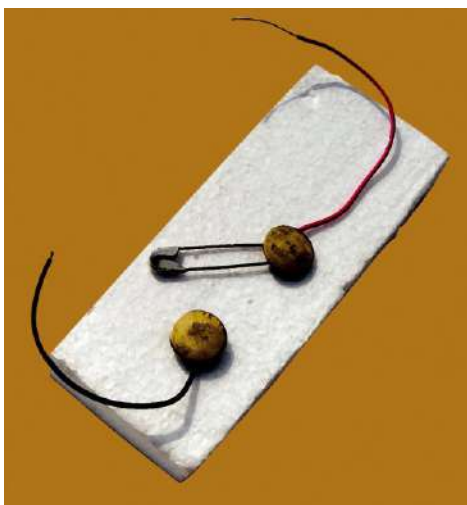
Figure 12.12 An Electric switch
