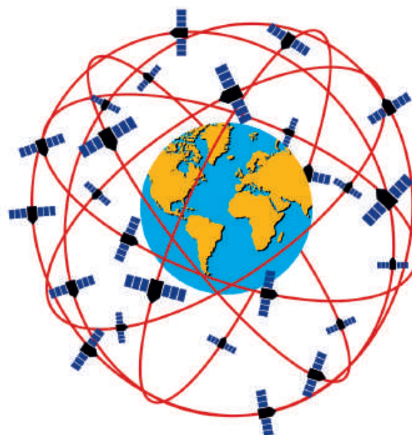
Figure 10.10 Constellation of GPS satellites around Earth
