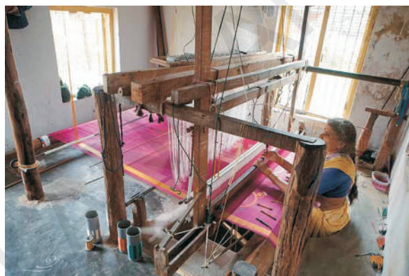
Fig. 9 A Jamdani sari on loom. Weft being woven over warp.
