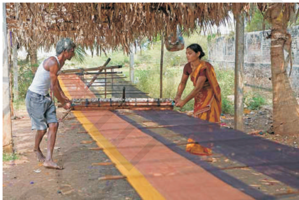
Fig. 8 Warp of sari being prepared.
