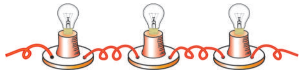
Fig. 12 - Bulbs connected in series
