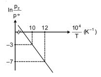
$(\text{Given, } \frac{\text{d(ln K)}}{\text{d}\left(\frac{1}{T}\right)} = -\frac{\Delta H^e}{R} \text{, where the equilibrium constant, } K = \frac{p_z}{p^e} \text{ and the gas constant, } R = 8.314 \text{ J K}^{-1} \text{ mol}^{-1})$
