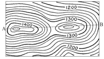
Fig. 3 : Ridge and saddle (AB is the ridge line)
