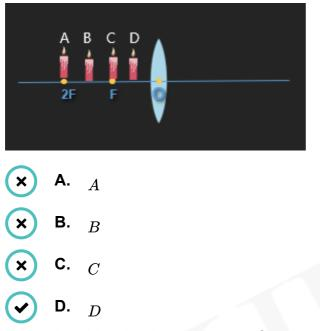
When the object is placed between focus and optical center, the image formed is virtual, erect and enlarged. So, the candle should be placed at A.
