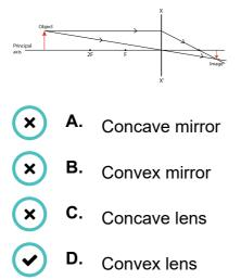
This is a convex lens. The rules of ray diagrams for image formation are followed similar to that of a convex lens, as shown.
