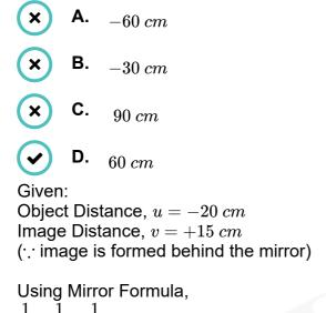
$\frac{1}{u} + \frac{1}{v} = \frac{1}{f}$   $\frac{1}{-20} + \frac{1}{15} = \frac{1}{f}$   $f = +60 \ cm$ Since *f* is positive, mirror used here is convex mirror.
