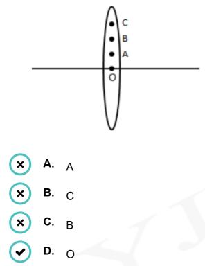
For a thin convex lens, the light ray passing through the optical centre would pass undeviated. The optical centre is represented by O in the given image.
