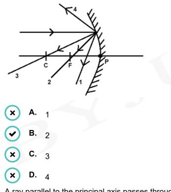
A ray parallel to the principal axis passes through the focus after reflection from a concave mirror as shown.
