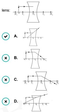
A light ray coming from an object and running parallel to the principal axis of the lens gets diverged after passing through a concave lens. The ray when traced back seems to originate from the virtual focus of the lens as shown in the figure :
