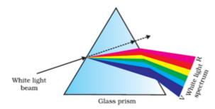
The refractive index of the medium is maximum for the violet light and minimum for the red light. Therefore, when white light enters a prism, it disperses into seven constituent colours and violet light shows the maximum deviation.
