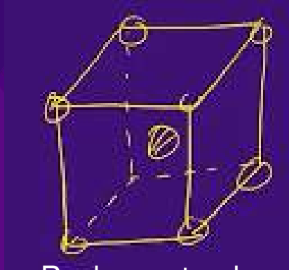
Body-centred cubic unit cell
