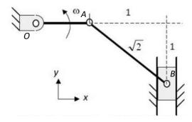
Velocity of point A,  $V_A = r \times \omega$
