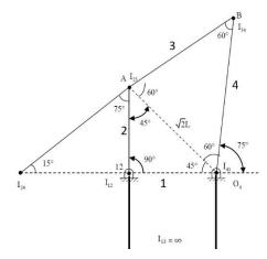
$$I_{24}I_{12}\omega_2 = I_{24}I_{41}\omega_4$$
