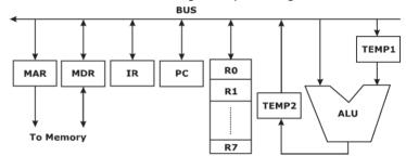
Consider an instruction:  $R0 \leftarrow R1 + R2$ . The following steps are used to execute it over the given data path. Assume that PC is incremented appropriately. The Subscripts r and w indicate read and write operations, respectively.
