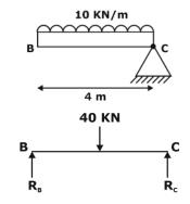
Moment at B  $40 \times 2 = R_C \times 4$  $R_C = 20 \text{ kN}$
