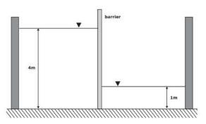
Taking the density of water as 1000 kg/m<sup>3</sup>, and the acceleration due to gravity as 10 m/s<sup>2.</sup> The maximum absolute bending moment developed in the cantilever is kN.m (round off to the nearest integer).
