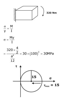
$\tau$  = 15 MPa which is less than shear strength of material
