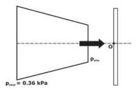
The inlet and outlet areas of the nozzle are 0.1  $m^2$  and 0.02  $m^2$ , respectively. Take air density as constant and equal to 1.2 kg/m<sup>2.</sup> If the inlet gauge pressure of air is 0.36 kPa, the gauge
