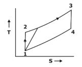
For above (T-S) diagram of Brayton cycle, Isentropic efficiency ( $\eta_{isen}$ ) = 0.85
