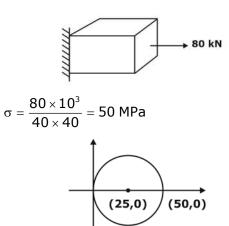
$\tau_{max}$  = 25 MPa which is greater than shear strength of material
