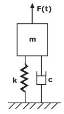
The non-zero value of  $\omega$ , for which the amplitude of the force transmitted to the ground will be F<sub>0</sub>, is
