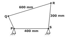
For the mechanism to be a crank-rocker mechanism, the length of the link PQ can be
