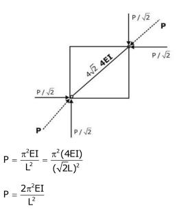
40. Bars of square and circular cross-section with 0.5 m length are made of a material with shear strength of 20 MPa. The square bar cross-section dimension is 4 cm × 4 cm and the cylindrical bar cross-sectiondiameter is 4 cm. The specimens are loaded as shown in the figure.
