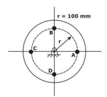
The rotor is driven by a motor at uniform angular speed of 10 rad/s. If one of the masses gets detached then the magnitude of the resultant unbalance force on the rotor is
