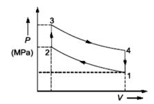
$$P_1 = 0.1 \text{ MPa, } T_1 = 35^{\circ}C = 308 \text{ K}$$
