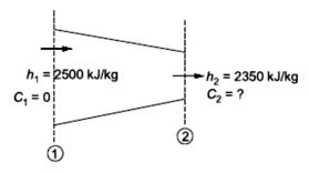
$\dot{m} = 0.1 \text{ kg/s}, \ Q = 5 \text{ kW (heat loss)}$
