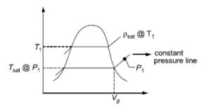
P<sub>1</sub>, T<sub>1</sub> represent the state of superheated vapours.
