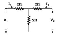
The parameter B for the given two-port network (in ohms, correct to two decimal places) is
