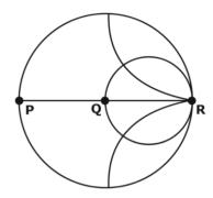
A. P : Open Circuit, Q : Short Circuit, R : Matched Load
