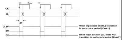
Now average voltage at node X can be calculated according to the timing diagram,
