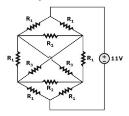
The magnitude of the current (in amperes, accurate to two decimal places) through the source is \_\_\_\_\_\_.
