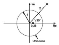
For the system to be stable, ROC should include the unit circle. From the given pole pattern, it is clear that to make the system stable, the ROC should be two-sided and hence the impulse response of the system should be also two-sided.
