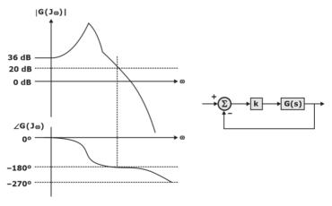
Consider the negative unity feedback configuration with gain k in the feedforward path. The closed loop is stable for  $k < k_0$ . The maximum value of  $k_0$  is
