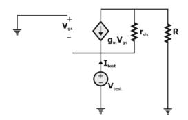
$$V_{test} = -V_{qs}$$
