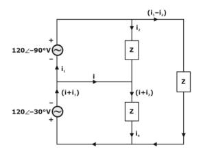
$$i_2 = \frac{120 \angle - 90^{\circ}}{Z} = \frac{120 \angle - 90^{\circ}}{(80 - 35j)}$$
