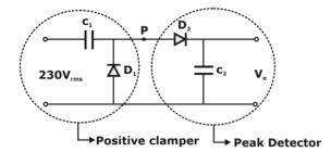
So the peak value at 'P' m 2Vm, Then the voltage across  $C_2$  which is  $2V_m$ .
