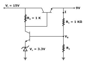
Voltage  $V_B = V_z + V_{BE}$ = 3.3 + 0.7
