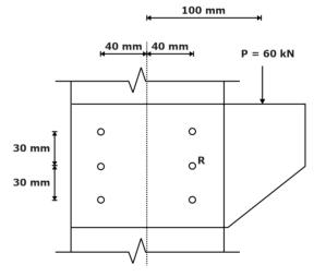
The resultant force in bolt R (in kN, round off to one decimal place) is \_\_\_\_\_.
