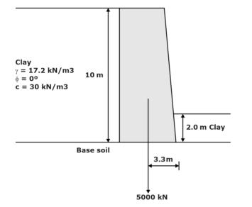
The factor of safety (round off to two decimal places) against sliding failure of the retaining wall after ignoring the passive earth pressure will be\_\_\_\_\_.
