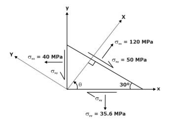
The absolute magnitude of the shear stress component  $\sigma_{xy}$  (in MPa. round off to one decimal place) in x-y coordinate system is \_\_\_\_\_.
