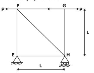
If R =  $500 \times 10^3$  kN, P= 150 kN and L = 3 m, the magnitude of the horizontal displacement of joint G (in mm. round off to one decimal place) is \_\_\_\_\_.
