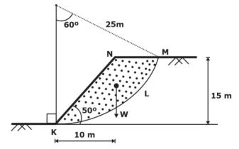
Considering the trial slip circle KLM, the factor of safety against the failure of slope under undrained condition (round off to two decimal places) is \_\_\_\_\_.
