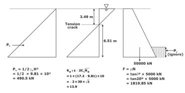
Depth of tension crack =
