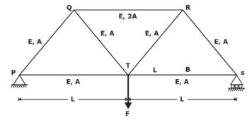
If load, F = 10  $\sqrt{3}$  kN, moment of inertia, I= 8.33 = 10<sup>6</sup> mm<sup>4</sup>, area of cross-section, A = 10<sup>4</sup> mm<sup>2</sup> and length, L = 2 m for all the members of the truss, the compressive stress (in kN/m<sup>2</sup>, in integer) carried by the member Q-R is \_\_\_\_\_.
