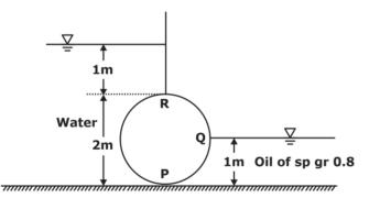
The absolute ratio of the net magnitude of vertical forces to the net magnitude of horizontal forces (round off to two decimal places) is \_\_\_\_\_.
