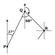
Given, FB of PQ = 27° ∴ BB of PQ = 180 + 27 = 207 ∴ FB of QR = B.B. of PQ - 68° = 207 - 68 = 139° ∴ BB of QR = 180 + 139 = 319° ∴ FB of RS = BB of QR - 123° = 319 - 123 = 196° The shape of the most commonly
