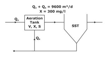
Solid loading to SST =  $(Q_0 + Q_R) x =$   $\frac{6900}{24} \frac{m^3}{h} \times \frac{3000 \times 10^{-6}}{10^{-3}} \frac{kg}{m^3}$ Solid flux = 3.2 kg/m<sup>2</sup>.h = 1200 kg/h Surface area of SST =  $\frac{1200 \text{ kg}/\text{h}}{3.2 \text{ kg/m}^2.\text{g}} = 375 \text{ m}^2$
