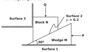
The limiting force P, in terms of Q, required for impending motion of block N to just move it in the upward direction is given as P = aQ. The value of the coefficient 'a' (round off to one decimal place) is
