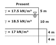
$$\overline{\sigma}_{\text{Present}} = 17.5 \times 5 + 10 \times (18.5 - 9.81) + 4 \times$$
