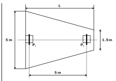
If the stress beneath the footing is uniform, the length of the combined footing L (in m, round off to two decimal places) is \_\_\_\_\_.
