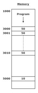
At address 1004, the second instruction is present. Instruction from  $2^{nd}$  to  $7^{th}$  are in loop, loop will be terminated when  $R_1$  becomes zero. In the first iteration value at address "3000" will be 60.
