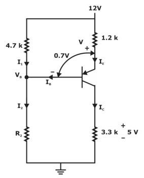
$$\begin{split} R_2 &= \frac{V_B}{I_2} \\ I_c &= \frac{5}{3.3} = 1.515 \text{ mA} \\ I_B &= \frac{I_C}{B} = \frac{1.515}{100} \text{mA} = 0.0151 \text{ mA} \\ I_E &= I_c + I_B = 1.530 \text{ mA} \\ V_B &= 12 - 1.2 \text{ I}_E - 0.7 \\ V_B &= 9.46V \\ I_2 &= I_1 + I_B = \frac{12 - 9.46}{4.7} + \frac{1.515}{100} = 0.55 \text{ mA} \\ R_2 &= \frac{9.46}{0.550} = 17.02 \text{ k}\Omega \end{split}$$
