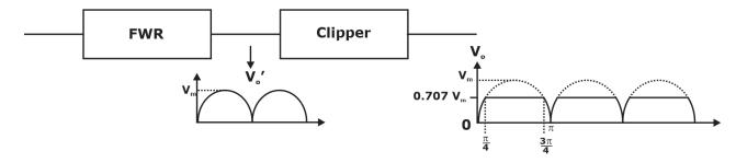
$$V_{\text{rms Clipped}} \ = \left[\frac{1}{\pi} \int_0^{\frac{\pi}{4}} V_m^2 \, \sin^2\theta \cdot d\,\theta + \int_{\frac{\pi}{4}}^{\frac{3\pi}{4}} \left(\frac{V_m}{\sqrt{2}}\right)^2 \cdot d\,\theta + \int_{\frac{3\pi}{4}}^{\pi} V_m^2 \, \sin^2\theta \cdot d\,\theta\right]^{\frac{1}{2}}$$
