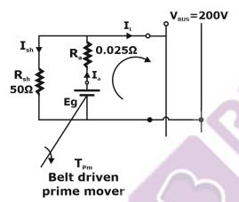
The machine starts consuming 10 kW Power due to absence of mechanical input.
