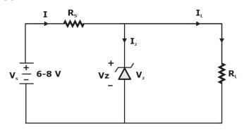
$$I_{z \text{ Mininum}} = I_{\text{Mininum}} - I_{\text{L Maximum}} \ge I_{\text{zk}}$$
