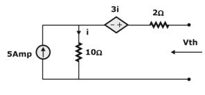
$$V_{th} = V_{ab} = 2 \times 3i + 10i$$
