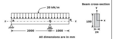
The maximum bending stress developed in the beam is \_\_\_\_\_ MPa (round off to one decimal place).
