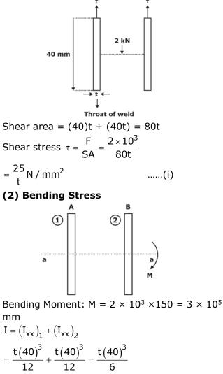
$$\sigma_{b} = \frac{3 \times 10^{5}}{\frac{t \times (40)^{3}}{6}} \times 20 = \frac{562.5}{t} \dots$$
