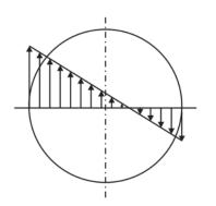
The shear stress distribution given represents Combined direct shear stress in the coil wire Cross-section.
