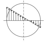
A. torsional shear stress in the coil wire crosssection
