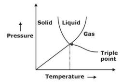
At triple point liquid vapour line and solid vapour line will coincide
