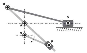
The quick return ratio for the mechanism is \_\_\_\_\_ (round off to one decimal place).
