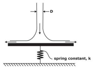
If the spring shows a steady deflection of 1 cm upon impingement of jet, then the velocity of the incoming jet is \_\_\_\_\_ m/s (round off to one decimal place).
