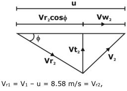
$$V_{w2} = u - V_{r2} \cos \varphi = 23.12 \text{ m/s},$$
