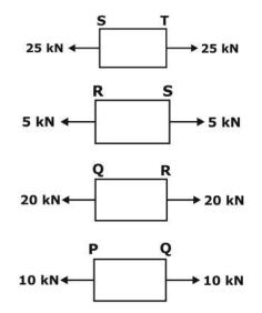
The max load of 25 kN is on `ST' Portion, Hence  $\sigma_{\text{ST}}$  = Max stress
