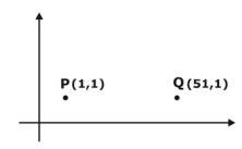
As motion between point P and Q is (51 - 1) =50 mm
