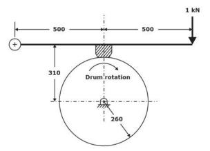
The magnitude of the torque applied by the brake is \_\_\_\_\_ Nm(round off to one decimal place).
