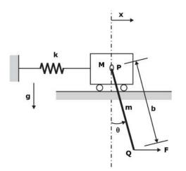
Assume that the spring deflects only horizontally and force F is applied horizontally at Q. For this system, the Lagrangian, L is
