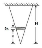
Consider an elementary section of length  $\delta x$ , at a distance x from the free end.
