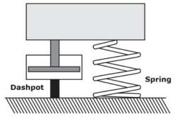
If the amplitude of the free vibration response reduces from 8 mm to 1.5 mm in 3 cycles, the damping ratio of the system is \_\_\_\_\_ (round off to three decimal places).
