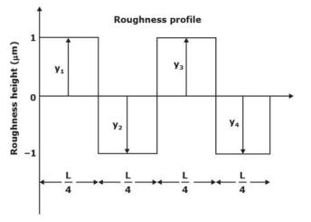
The center line average roughness ( $R_a$ , in  $\mu m$ ) of the measured length (L) is
