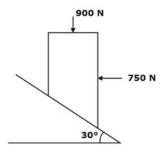
The coefficient of static friction between the block and surface is \_\_\_\_\_\_ (round off to two decimal places).
