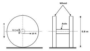
Each wheel has diameter 0.8 m and mass 1 kg. Assume that the mass of the wheel is concentrated at rim and neglect the mass of the spokes. The diameter of axle is 0.2 in and its mass is 1.5 kg. Neglect the moment of inertia of the axle and assume g = 9.8 in  $s^{B.}$  An effort of 10 N is applied on the axle in the
