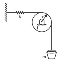
The pulley radius is r and its mass moment of inertia is J. Assume the mas is vibrating harmonically about is equilibrium position. The frequency natural of the system
