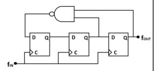
A. It can be used for dividing the input frequency by 3.
