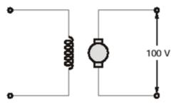
Producing a torque of 500 N-m At zero speed, N = 0 and E<sub>b</sub> = 0 and E<sub>b</sub> = V<sub>t</sub> - I<sub>a</sub>r<sub>a</sub>  $I_a = \frac{V_t}{r_a} = \frac{100}{0.05} = 2000A$ Since T = K<sub>a</sub> $\phi$ I<sub>a</sub> K<sub>a</sub> $\phi = \frac{500}{2000} = \frac{1}{4}$
