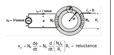
$$\begin{split} v_{p} &= \frac{N_{p}^{2}d\left(I\sin\omega t\right)}{dt} = \frac{N_{p}^{2}}{R_{1}}\,\omega I\cos\omega t = V\cos\omega t\\ V &= \frac{N_{p}^{2}\omega I}{R_{1}} = \frac{N_{p}^{2}\omega I}{I} = \frac{\mu N_{p}^{2}\omega IA}{I} = \frac{\mu N_{p}^{2}\omega I\pi r^{2}}{2\pi R}\\ \text{Hence, } R &= \frac{\mu Ir^{2}N_{p}^{2}\omega}{2V} \end{split}$$
