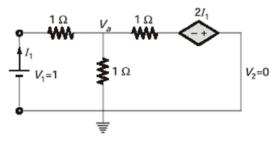
$$\begin{split} &\frac{V_{a}-1}{1}+\frac{V_{a}}{1}+\frac{V_{a}+2I_{1}}{1}=0\\ &3V_{a}+2I_{1}=1\quad\ldots.(i)\\ &I_{1}=\frac{1-V_{a}}{1}\qquad\ldots.(ii) \end{split}$$
