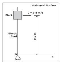
The cord hinged at O is initially unstretched and always remains elastic. The block is given a velocity v of 1.5 m/s perpendicular to the cord. The magnitude of velocity in m/s of the block at the instant the cord is stretched by 0.4 m is
