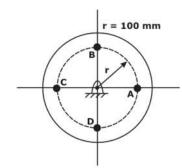
The rotor is driven by a motor at uniform angular speed of 10 rad/s. If one of the masses gets detached then the magnitude of the resultant unbalance force on the rotor is \_\_\_\_\_\_ N (round off to 2 decimal places).
