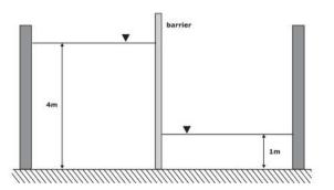
Taking the density of water as 1000 kg/m<sup>3</sup>, and the acceleration due to gravity as 10 m/s<sup>2.</sup> The maximum absolute bending moment developed in the cantilever is kN.m (round off to the nearest integer).
