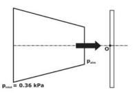
The inlet and outlet areas of the nozzle are 0.1  $m^2$  and 0.02  $m^2$ , respectively. Take air density as constant and equal to 1.2 kg/m<sup>2.</sup> If the inlet gauge pressure of air is 0.36 kPa, the gauge pressure at point O on the plate is \_\_\_\_\_\_ kPa(round off to two decimal places).
