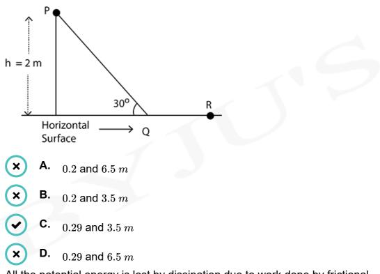
All the potential energy is lost by dissipation due to work done by frictional force.
