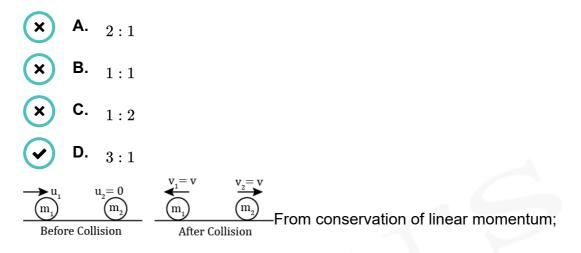
$egin{aligned} p_i &= p_f \ &\Rightarrow m_1 u_1 + m_2(0) = m_1(-v) + m_2 v \ &\Rightarrow m_1 u_1 = v(m_2 - m_1) \quad \dots \dots (i) \end{aligned}$
