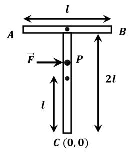
To have translational motion without rotation, the force  $\overrightarrow{F}$  has to be applied at COM that lies on 'P' Taking point C at the origin
