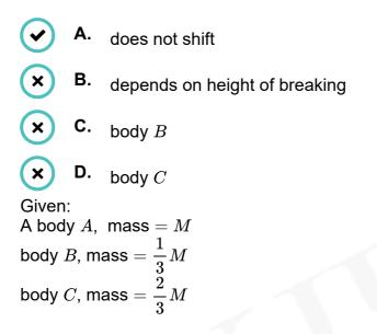
The centre of mass of bodies B and C taken together does not shift as no external force acts.
