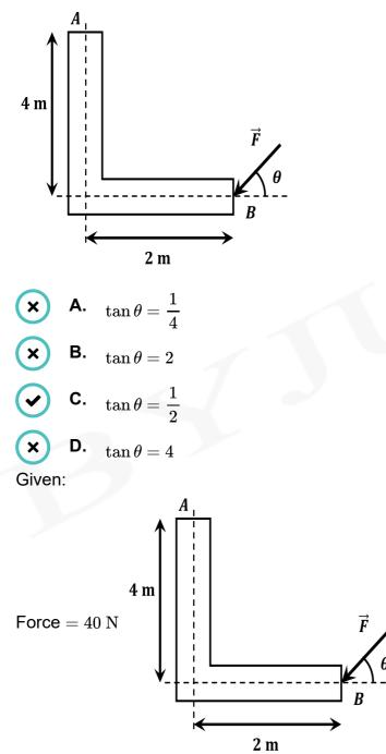
To produce maximum moment of force line of action of force must be perpendicular to line AB.
