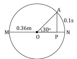
The point  $A \text{ covers } 30^\circ \text{ in } 0.1 \text{ s.}$ From unitary method it means,
