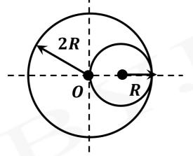
The mass of the removed disc  $= \sigma(\pi R^2) = \pi \sigma R^2$
