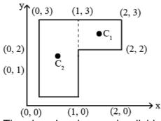
The given Lamina can be divided into two parts, as shown.
