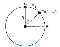
Particle crosses the point B but not complete the vertical circle. Tension will be zero in between B to C & the angle where T = 0
