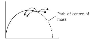
**Explanation.** The projectile follows a parabolic path under the action of gravity (i.e. earth's gravitational force) Explosion of the projectile occurs due to the internal forces i.e, without any external force. These internal forces cannot change the total momentum of the system al though they may change the momenta of the individual fragments. Thus the centre of mass will remain unaffected after the explosion and hence follow the same parabolic path.
