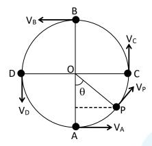
(c) If the body at point P has critical velocity for just completing vertical circle
