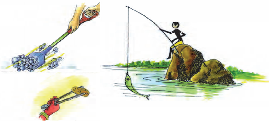
Fig. 11.11 Lever of the Third kind
