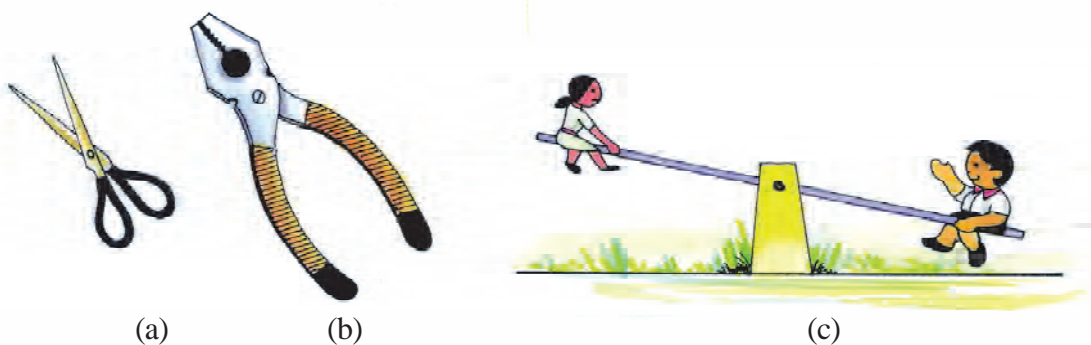
Fig. 11.9 Lever of the First kind
