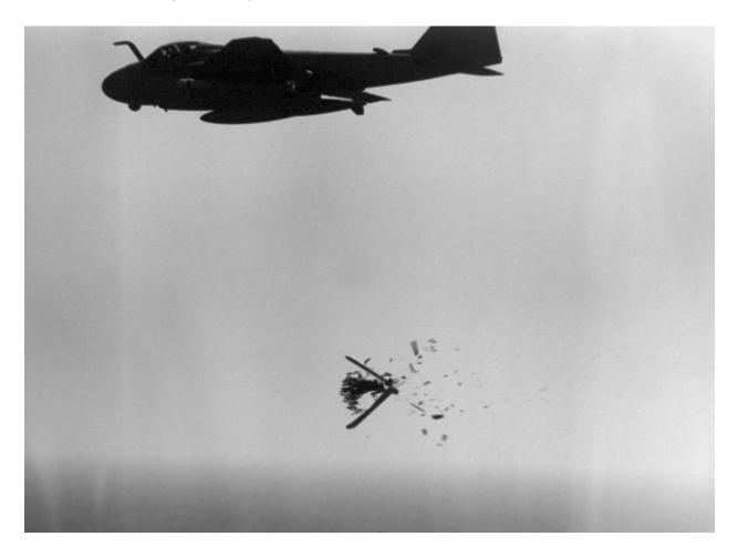
An example of a cluster munition being dropped from an aircraft. As seen in the picture, multiple submunitions are being released from a large bombshell.
