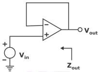
It has voltage series feedback. Output Impedance is given by
