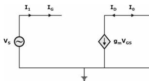
$$\mbox{Current gain = } \frac{I_{0}}{I_{i}} = \frac{-I_{D}}{I_{G}} = \frac{g_{m}V_{GS}}{0} = \infty \label{eq:current}$$
