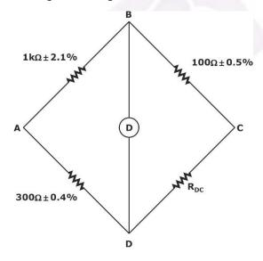
$$R_{\text{DC}} = \frac{R_{\text{AD}} \times R_{\text{BC}}}{R_{\text{AB}}}$$
