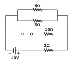
Voltage across 6  $\Omega$  is same as voltage across parallel combination of 6  $\Omega$  and 3  $\Omega$ .
