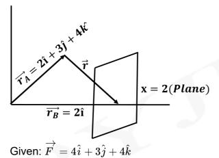
Position of intersection point where force is applied,  $\overrightarrow{r}_B = 2\hat{i}$ Point about which torque to be calculated,  $\overrightarrow{r}_A = 2\hat{i} + 3\hat{j} + 4\hat{k}$ Now, from figure  $\overrightarrow{r}_A + \overrightarrow{r} = \overrightarrow{r}_B$
