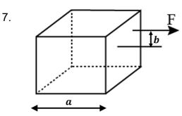
Consider a uniform cubical box of side 'a' on a rough floor that is to be moved by applying minimum possible force F at a point 'b' above its centre of mass (see figure). If the coefficient of friction is  $\mu = 0.4$ , the maximum possible value of  $100 \times \frac{b}{a}$  for the box not to topple before moving is .
