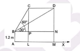
Then,  $(\angle CBP = 60^\circ, \angle DBN = 30^\circ, AB = PL = NM = 1.2 \text{ m})$  and (CL = DM = 88.2 m)
