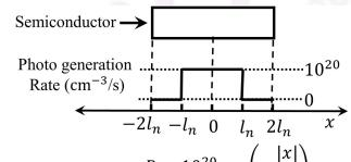
Excess minority carrier recombination rate (cm<sup>-3</sup>/s)  $R = 10^{20} \exp\left(-\frac{|x|}{l_n}\right)$   $10^{20}$
