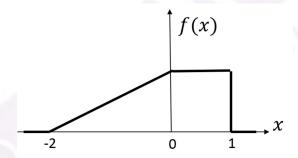
Consider a 1 bit quantizer that maps positive samples to value  $\alpha$  and others to value  $\beta$ . If  $\alpha^*$  and  $\beta^*$  are the respective choices for  $\alpha$  and  $\beta$  that minimize the mean square quantization error, then  $(\alpha^* - \beta^*) = \underline{\hspace{1cm}}$  (rounded off to two decimal places).
