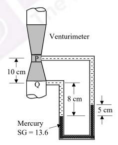
Taking specific weight of water as 9810 N/m<sup>3</sup>, the pressure difference (in Pa, rounded off to one decimal place) between point Q and P is
