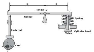
Resonance in the rocker system occurs when the cam shaft runs at a speed of rpm (round off to the nearest integer).
