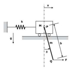
Assume that the spring deflects horizontally and force F is applied horizontally at Q. For this system, the Lagrangian, L is
