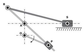
The quick return ratio for the mechanism is \_\_\_\_\_ (round off to one decimal place).
