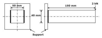
Considering that the allowable shear stress in weld is 60 N/mm<sup>2</sup>. The minimum size (leg) of the weld required is \_\_\_\_\_ mm (round off to one decimal place).
