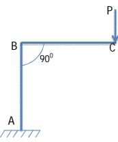
Q.17 Neglecting the axial compression of member AB, the deflection of point C in the direction of the load is
