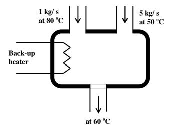
There is no accumulation of water in the tank. A back-up heater is provided to ensure a constant outflow temperature of water at  $60\,^{\circ}$ C from the tank under steady state. What is the required capacity of the back-up heater to the nearest kW?
