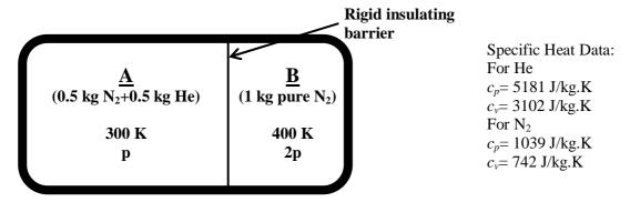
Initially, chamber A contains a mixture of 0.5 kg nitrogen and 0.5 kg helium at 300 K while chamber B contains 1 kg of pure nitrogen at 400 K. The pressure in chamber B is twice that in chamber A. The gases and gas mixtures are assumed to be ideal.
