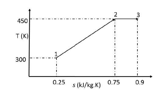
The "*T*-*s* diagram" for a thermodynamic process is shown in the figure. The heat transferred (**kJ/kg**) during the reversible process 1-3 is \_\_\_\_\_.
