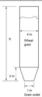
A circular grain silo with conical bottom, as shown in figure, is filled with wheat (true density 1200 kg m<sup>-3</sup>) with porosity of 0.6. Five hundred metric tonne of wheat fills 80% of its capacity (by volume). The total height (h) of the silo from its grain outlet end in m is \_\_\_\_\_\_\_.
