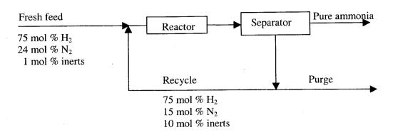
The single pass conversion for  $H_2$  in the reactor is 20 %. The amount of  $H_2$  lost in the purge as a **PERCENTAGE** of  $H_2$  in fresh feed is
