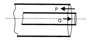
Densities of P and Q are 1000 and 800 kg/m³ respectively. The average velocities of the liquids P and Q are 1 and 2.5 m/s respectively. The inner diameters of the pipes are 0.31 and 0.1 m. Both pipes are 5 mm thick. The ratio of the Reynolds numbers Re<sub>P</sub> to Re<sub>O</sub> is
