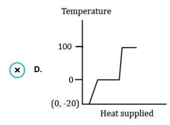
First, the ice at  $-20^{\circ}$ C converts to ice at  $0^{\circ}$ C, so there is constant increase in temperature. Thus, the graph will be a straight line starting from the origin, where the temperature is proportional to the Heat supplied.
