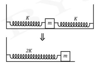
In a parallel combination, the equivalent spring constant is given by,  $K_{
