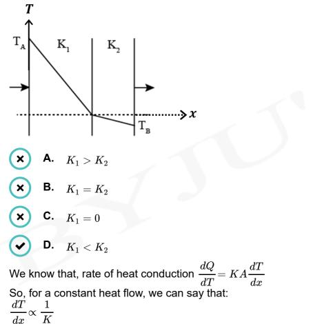
where  $\frac{dT}{dx}$  is the temperature gradient (slope of the lines in the figure) [As cross sectional area A is constant]
