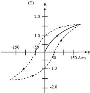
The figure gives experimentally measured B vs H variation in a ferromagnetic material. The retentivity, co-ercivity and saturation magnetization, respectively, of the material are:
