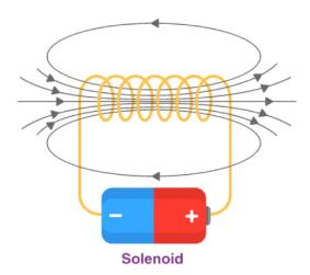
We can see from the figure that the magnetic field inside the solenoid is uniform in nature and is along the axis of the solenoid. The field at the exterior at any point immediately to the solenoid is very weak and the field lines cannot be seen near the close vicinity. It is important to note that the field inside it is parallel to its axis at every position.
