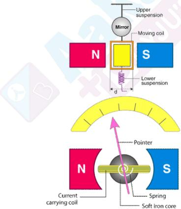
Moving coil galvanometer
