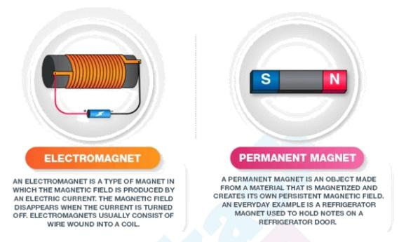
As the name suggests permanent magnet magnetic field is permanent and electromagnets magnetic field depends upon the flow of the electrical current. The electromagnet constitutes a coil made of wire which acts as a magnet when current is passed through it. Usually, a ferromagnetic material like steel is wrapped by an electromagnet to enhance its magnetic field.
