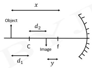
Distance of the object from the focus is :  $x = f + d_1$ Distance of image from the focus is :  $y = f - d_2$ Using Newton's formula for mirror :  $xy = f^2$   $(f + d_1)(f - d_2) = f^2$   $f^2 - fd_2 + fd_1 - d_1d_2 = f^2$  $d_1d_2$
