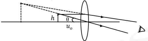
From the ray diagram, we can see that, the angular size of the object equals the angular size of the image  $(= \theta)$ .
