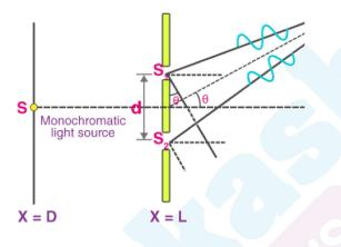
When the slit separation (d) and the screen distance (D) are kept unchanged, to reach P the light waves from  $s_1$  and  $s_2$  must travel different distances. It implies that there is a path difference in Young's double slit experiment between the two light waves from  $s_1$  and  $s_2$ .
