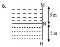
Two liquids of densities  $\rho_1$  and  $\rho_2$  ( $\rho_2 = 2\rho_1$ ) are filled up behind a square wall of side 10 m as shown in figure. Each liquid has a height of 5 m. The ratio of the forces due to these liquids exerted on upper part MN to that at the lower part NO is (Assume that the liquids are not mixing)
