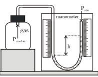
Excess Pressure  $(P - P_{atm})$  measured with the help of pressure measuring instrument called Gauge pressure.  $P_{gauge} = h\rho g$  or  $P_{gauge} \propto h$ Gauge pressure is always measured with help of **"manometer"**
