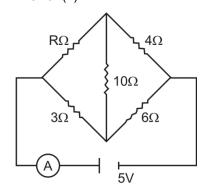
If Wheatstone bridge is balanced then current in 10  $\Omega$  resistor is zero.
