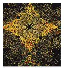
4.2 Field ion microscope image of iridium atoms (every spot in this image is an atom)
