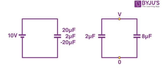
When battery is removed & the capacitor is connected
